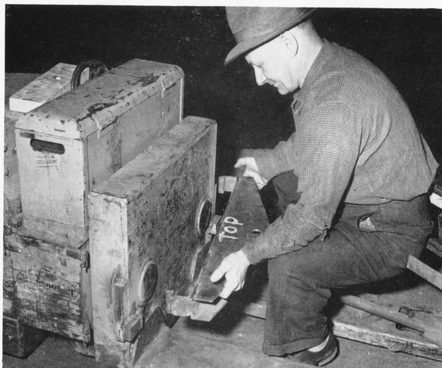
Arthur Boucher, Shipping and Receiving, demonstrates his award winning suggestion by adjusting a jig onto a small battery driven transporter which will enable it to accept the tongue of a freight wagon or other such apparatus.
